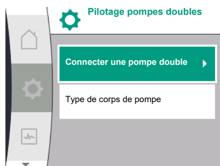
Fig. 49: Menu Pilotage pompes doubles
