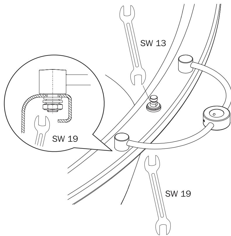
Fasten fixing devices with screws
