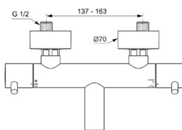
Technical drawing showing side view dimensions: top width 137 - 163 mm, top height Ø70 mm, and bottom height 20 mm.
